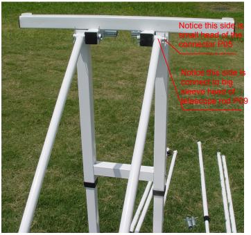
9: Connect diagonal rod supports to base leg and center plank. Used parts: #P05 and #P09 Notice the indication marked in picture
