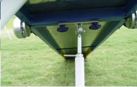
41-2. install the 2 ramp vertical support. Part # P08
