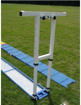
8: by pushing the snap peg heads on both sides of the leg to adjust dog walk to desired height.
