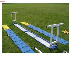
7: Repeat step 6 and tighten all knob screws to fix legs onto the center plank
