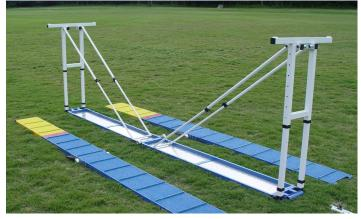
11: 4 sets of diagonal rods #P09 have been connected to the center plank and base legs
